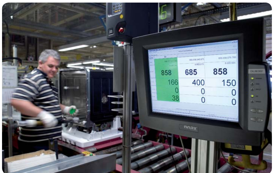
The steel enclosure will be a dishwasher, the noax IPC shows the job data
