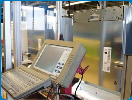
The high-voltage test is conducted by means of a noax IPC
