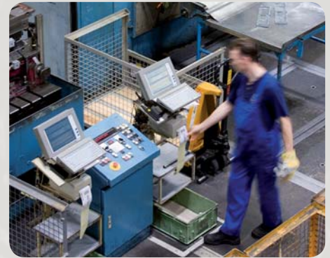
The printing order for bar code labels is controlled by a noax IPC
