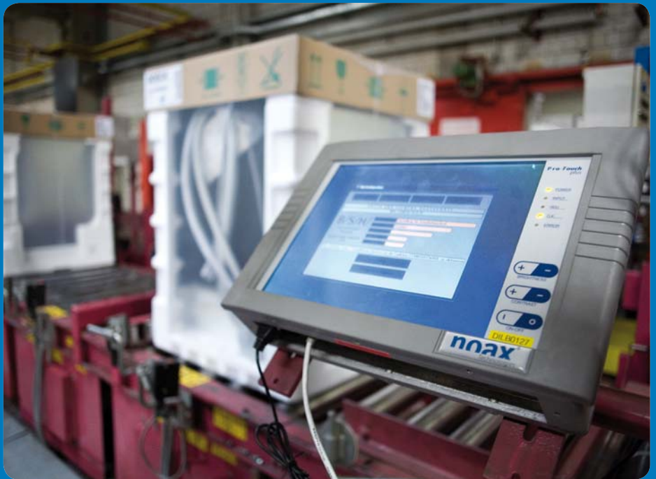
The noax IPCs log out dishwashers at three packaging lines, as they leave the assembly line
