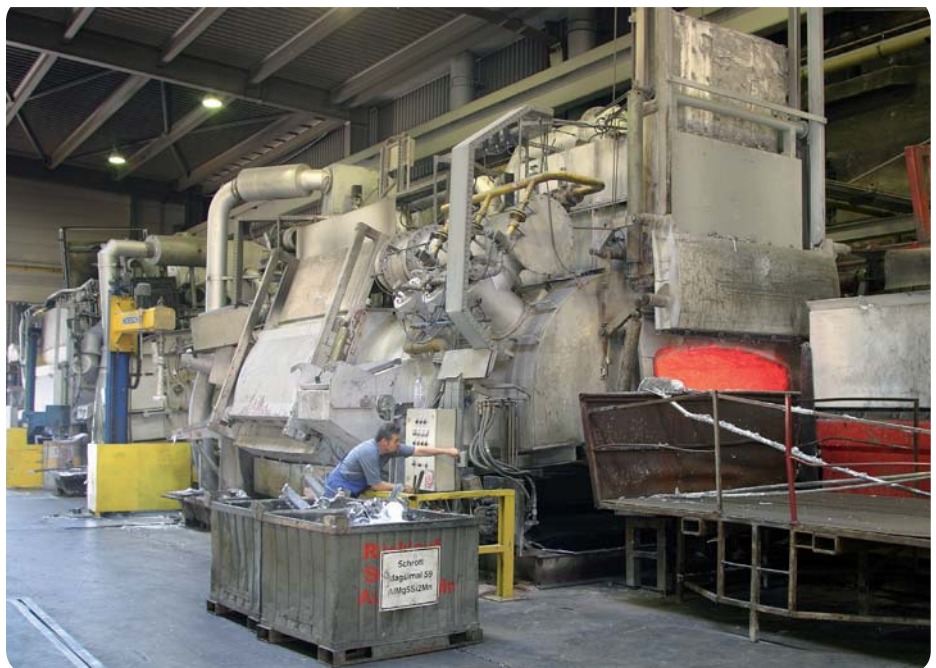
Aluminum smelting furnaces with a capacity of 10 to 20 tons
