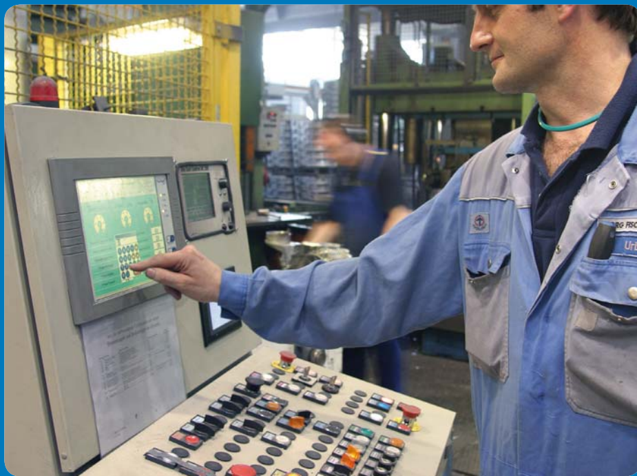
The completely sealed noax C12 rackmount pc installed in a control console
