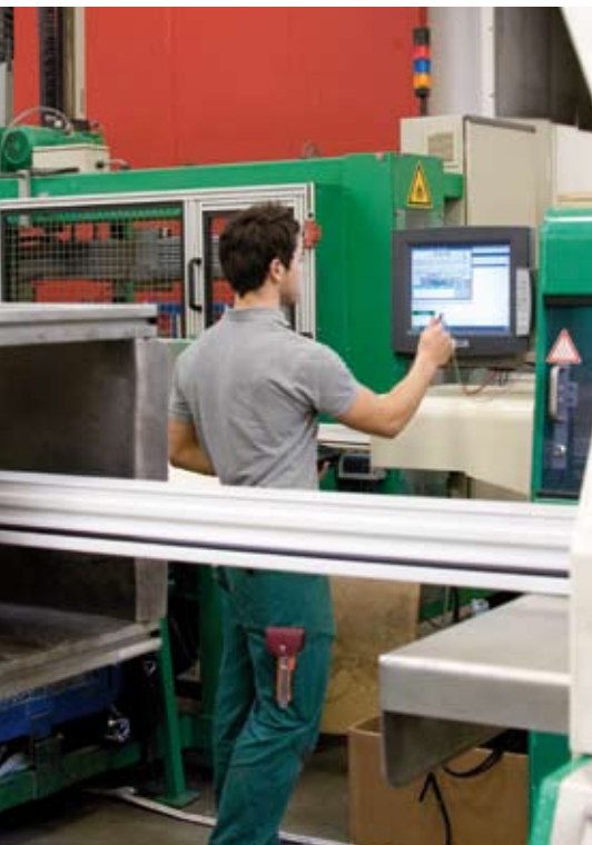
Using a noax IPC, an employee retrieves- MDA information.
