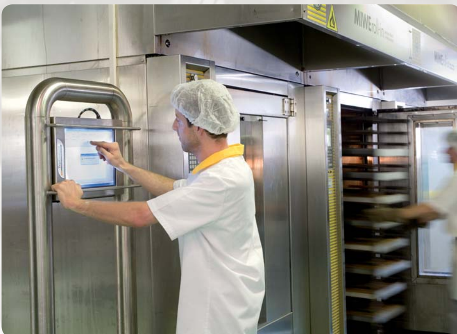
High-tech in the bakery: a noax IPC directly next to the oven controls baking times.
