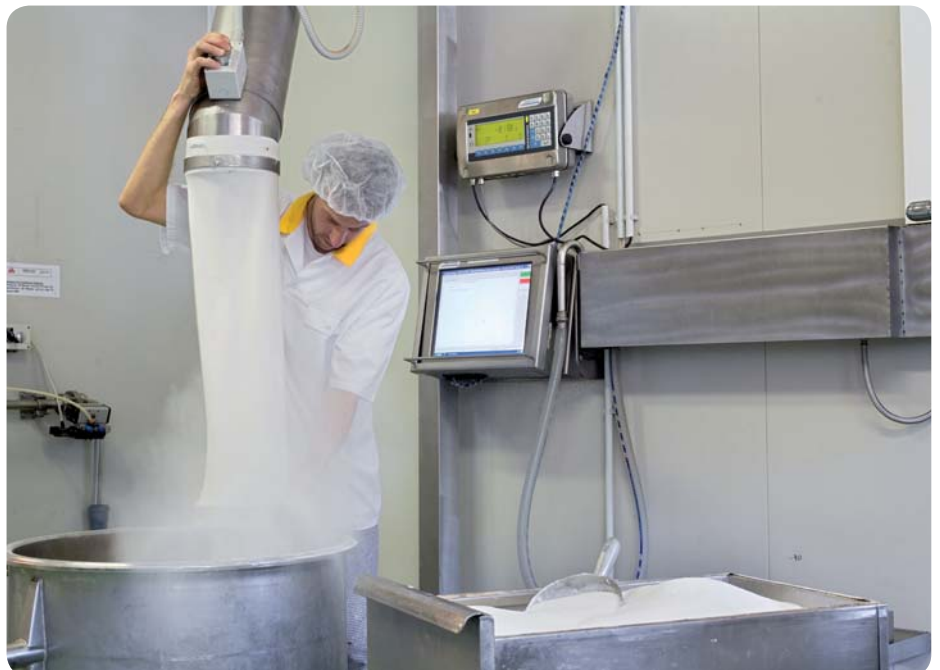
Completely sealed according to IP65. Flower dust does not affect the noax computer.
