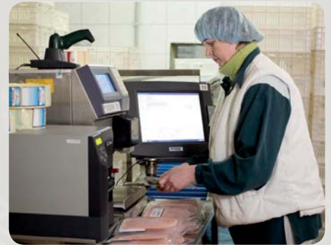
A noax IPC controls the label printing, as well as in-house logistics.
