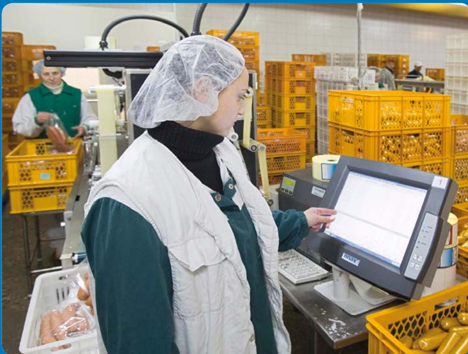
During in-house logistics, workers can be informed about the processing status of an order, by a noax IPC.
