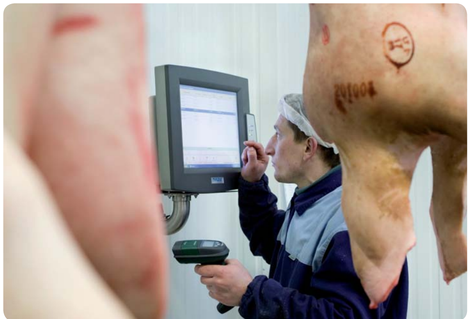
A worker scans the bar code labels, which are attached to pig halves. The data appears on a noax IPC and is entered into the product management system.
